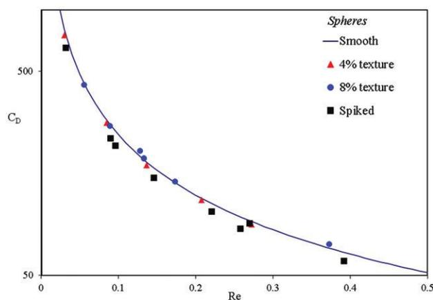
**Fig. 9** Effect of surface texture on drag of spheres. Drag coefficient ( $C_D$ ) versus Reynolds number ( $Re$ ) for four spheres. Types included smooth spheres, spheres with 4% texture (triangles), spheres with 8% texture (circles), and spheres containing conical “spikes” whose length was 12% of sphere diameter (squares). Surface texture does ultimately result in lower drag coefficients, but the effect does not become pronounced unless the texture is significant, as in spiked sphere.
